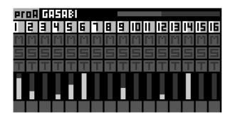
The icons **M** (mute), **S** (solo), **T** (temporary toggle), and **R** (multitrack recording) are showing the track states when highlighted:
