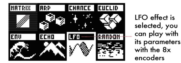
Use left screen and **Rotate** the 8x encoders to play with the selected effect parameters.
