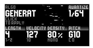
This algorithm replaces the existing notes with a new randomized pattern. Generated notes are quantized to the specified grid. The min & max pitch, velocity and length of the new notes can also be adjusted. Lastly, it is possible to set the amount of events (density %) and to decide whether the generated notes are monophonic or chords (mono ... poly 4).
