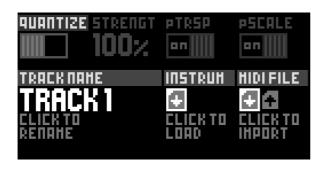
**Rotate** encoder ① to enable and set the rate of the quantizer. 1/16 is the coarsest setting, 1/64 is the most precise.
