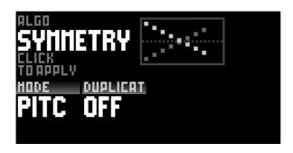
This algorithm flips events horizontally (time) or vertically (pitch). The original events can either be kept or replaced.
