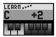
To turn **NOTE LEARN** off (and so stop the view moving when note are performed from an external controller), simply **Press** (or rotate) encoder ① or ②.
