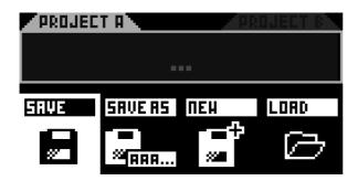
Note The SD card must be inserted to save or load projects.
