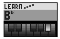
The pads are now reflecting notes played in **live** mode, or on an external keyboard. Playing a single note will move the view, so that the bottom row follows the note pressed.
