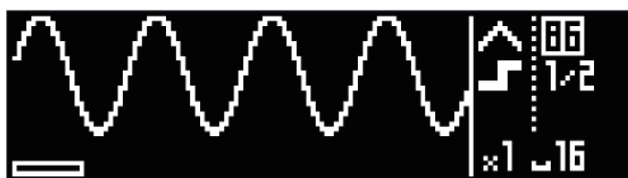
a sine wave modulation recorded from a CV input onto a mod track
