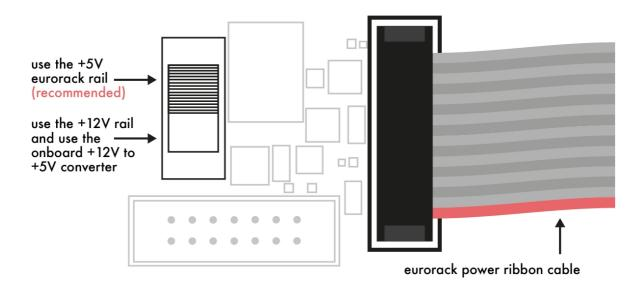
Note In any case, Hermod+ will not be damaged if you use the top position and your power supply does not deliver the +5V. It will simply not power up.
