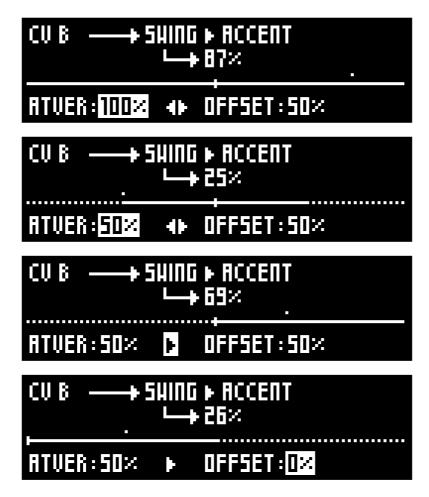
The horizontal dotted line displays the full modulation range available.
